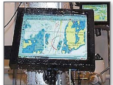
Locomarine SUB marine displays are fully submersible up to 1m of water depth.
